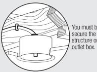
You must be able to secure the fan to building structure or fan-rated outlet box.
