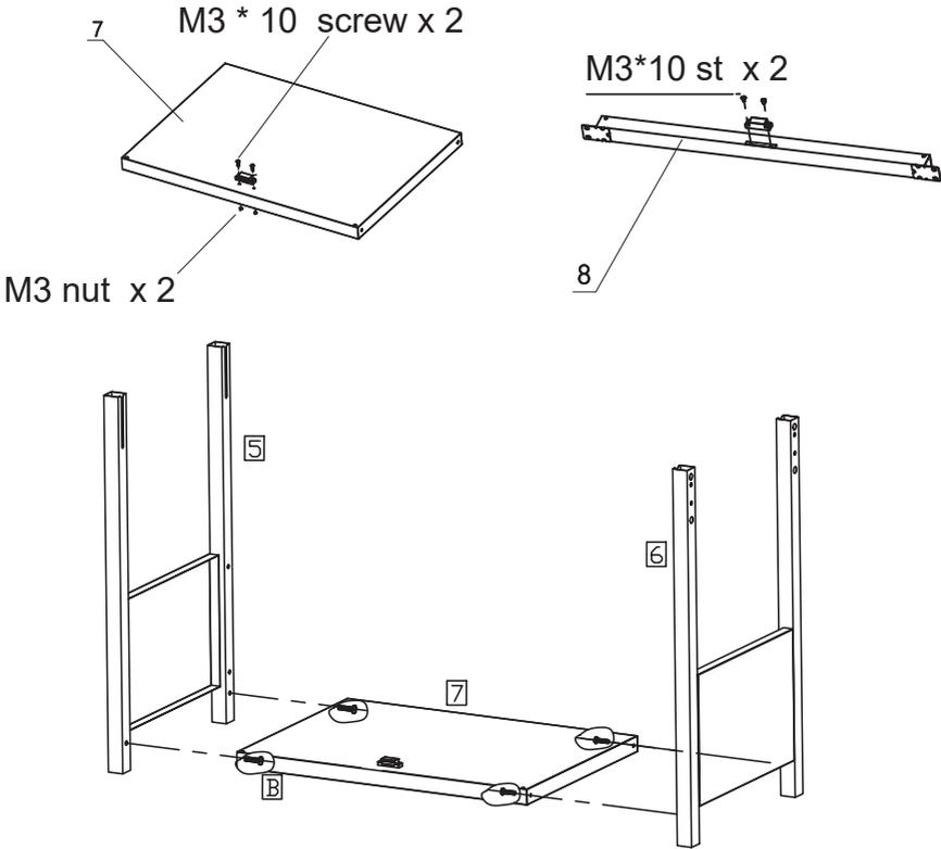
1. Assemble the LH and RH frame (5&6) to bottom shelf (7) with 4pcs M5 screws (B).
