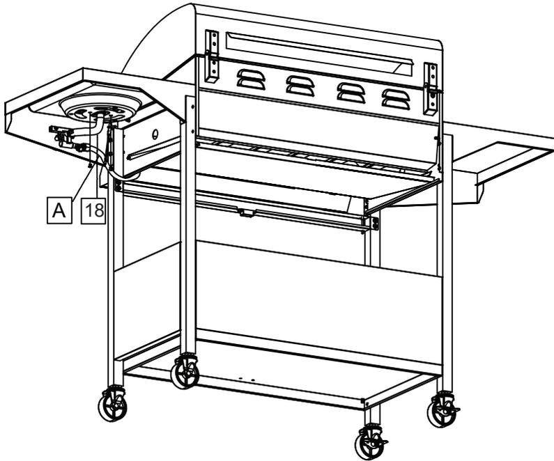
9-1. Side burner (18) is assembled into the side burner shelf with 2 pcs M4 screws (A). Insert the tube to valve connector.
