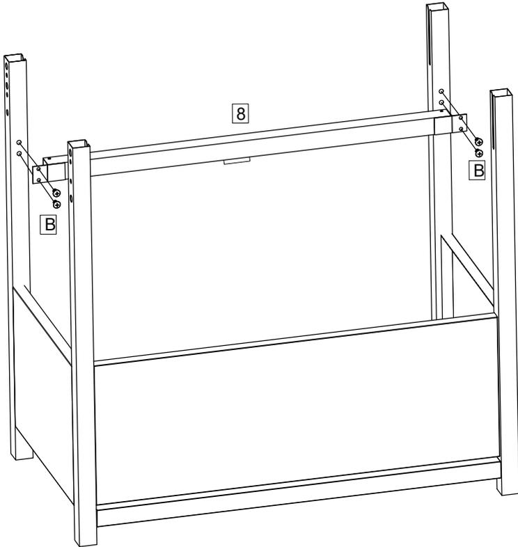
3. Assemble the front beam (8) to the front of frames with 4pcs M5 screws (B).
