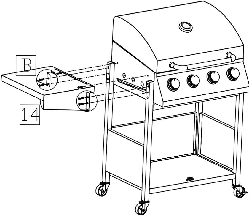
6. LH side shelf (14) is assembled to the body with 6 pcs M5 screws (B).
