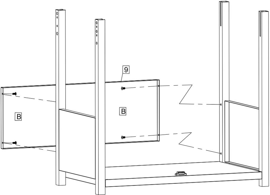
2. Assemble the back shelf (9) to the frames with 4 pcs M5 screws (B).
