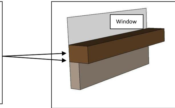
Our product is designed to allow natural movement that protects from freezing, thawing, and settling. If you use adhesive on the Adorn panels, only place in the noted area to allow for drainage.
