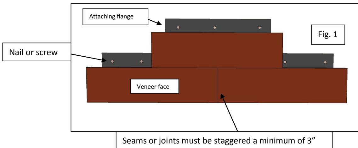
If the project requires corners, install the corner first and work out on both sides. Corners should be installed with each course. Each corner piece needs two screws or nails to securely attach. Inside corners use the same corner pieces reversed.
