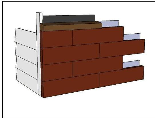
To finish projects where Adorn is to be installed up to the soffit, measure the distance from the last full panel installed to the soffit. Cut Adorn panels to fit and glue into place using construction adhesive, such as PL Premium. You may need to trim the attaching flange from the last full panel or securely attach a non-painted, clean flashing material to the structure to achieve a good bond surface.
