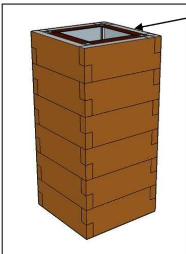
When you get to the top course, bend the flashing over the frame and screw in place.
