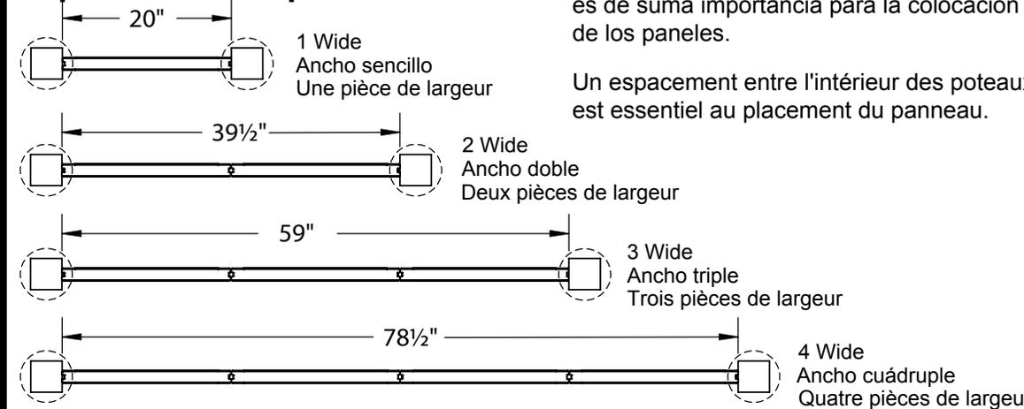
Spacing between inside of posts is critical for Panel placement.
