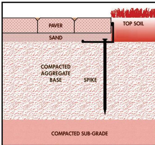
Anchoring tabs facing away from the pavers, with outer edging wall against pavers and sand, and tab under topsoil
