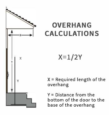
**For example,** if the measurement from the base of the door to the bottom of the overhang is 8 feet, then the required overhang length is 4 feet.
