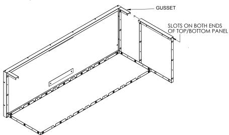
Step 5: Secure top panel to side and back panels using (4) M4 screws through pre-drilled holes and into gussets.
