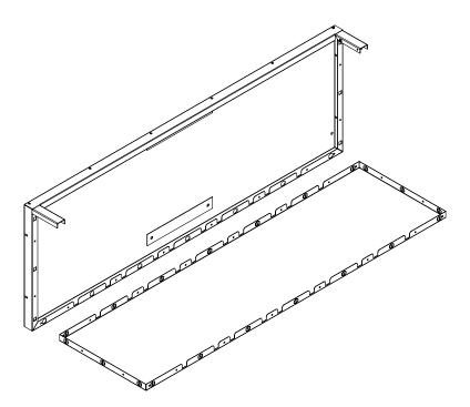
Step 3: Align holes and secure side panel using the pre-drilled holes and (8) M4 machine screws.
