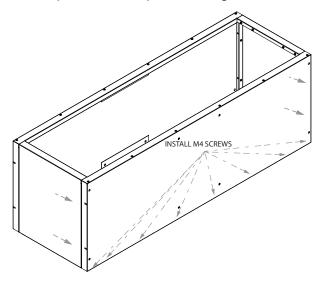
Step 8: Locate the two Reinforcing Channels. Place a Reinforcing Channel into the Gusset in the top panel. Secure with (2) M4 screws at each end of the Reinforcing Channel. Repeat procedure for the bottom panel.
