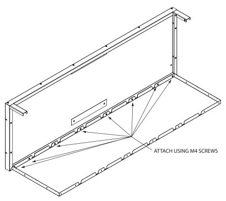
Step 4: Slide top/bottom panels through the slots and onto the gussets of the side panel.
