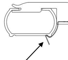
Insert screwdriver here and gently pry to release.
