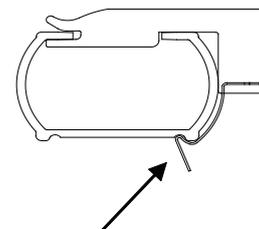
Insert screwdriver here and gently pry to release.
