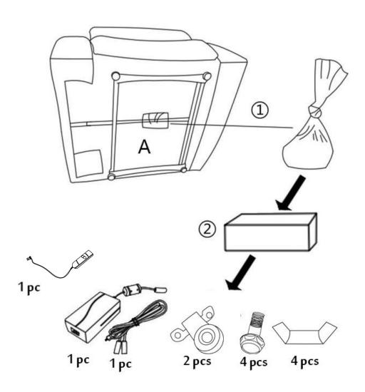
Place the main seat (A) on it's back, and fixing the two Anti-Skid and Anti-Scrape Feet with bolts as below:
