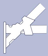
3. Use screws to mount bracket on a vertical or horizontal surface. Insert pole into bracket.
