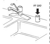
that the drain hose either be looped up and securely fastened to the underside of the counter, or be connected to an air gap.
