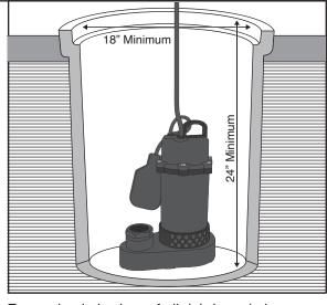
Ensure basin is clear of all debris and place pump on hard level surface (not dirt or gravel). 18" x 24" minimum basin size required.
