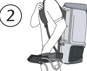
Loosen the shoulder straps and the waist belt. Lift the vacuum and slide your arms through the straps.
