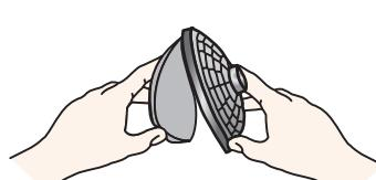
Pull the top piece of the Dome Filter off and remove the foam media. Shake it out, rinse it, and let it AIR dry thoroughly.
