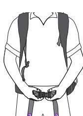
Connect the waist strap. Tighten the waist belt by grabbing the ends of the straps and pulling them toward each other and then directly outward from the center of the body. It is very important that the weight of the unit be concentrated on your hips rather than your shoulders.
