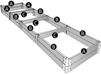
**STEP 6**: Insert a stake through the brackets into the hole on the top of the stake beneath it to lock the 2<sup>nd</sup> level in place.
