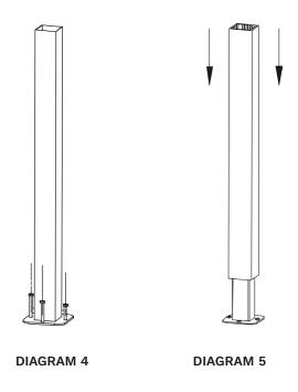
4 First, mark on the post which will be on the stair top using the "Stairs - Top Post" cardboard template. Use the top 4 holes for top post brackets and use the bottom 2 holes for the bottom post brackets.
