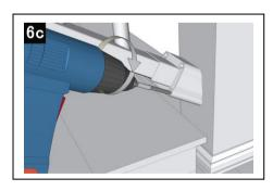
6c. Attach bottom stair rail stair bracket to lower post using two #3-15/16" wood screws and two #5-1/2" wood screws (provided). For best results set drill to low speed when installing these screws.
