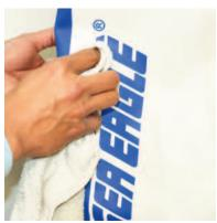
Once you have located the leak make sure you thoroughly clean the area surrounding the leak of any dirt or grime. After the area is clean and dry you can circle the area to make locating the leak easier throughout the repair process.
