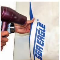
Use a hair dryer on the high setting to activate the adhesive and from there you can press firmly on the patch until cooled. It is VERY IM-PORTANT that you DO NOT use a hair dryer on an inflated boat.
