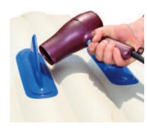
Using a hair dryer, warm up the skeg until the curve becomes soft. This should only take a about 2-3 minutes on a normal setting. Once the skeg(s) is soft you can then straighten it out by hand.
