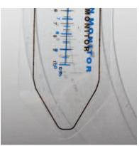
Inflate the three main chambers of the hull and the bow and stern spray skirts. You can safely inflate up to 1 centimeter beyond the diagram. When the boat is fully inflated you should be able to indent your thumb into the material about 1/2 to 3/4 of an inch.
