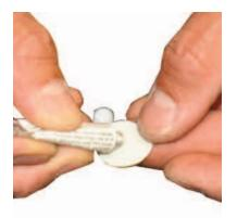
Apply adhesive to the dull side of the patch and around the area to be repaired. Coat the affected area lightly but completely with glue.
