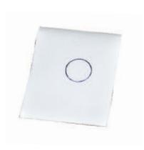
Using a ball point pen, trace the outline of your patch which should be large enough to overlap the damaged area by approximately 1/2". Angle the pen inward a bit so that the ink will be covered by the patch later.
