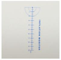
Printed on the inside of your kayak is a diagram of the plastic inflation monitor that is included with this boat. As you begin to inflate, the hull material will stretch so that the printed diagram will expand to match the clear plastic inflation monitor.
