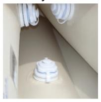
To begin unroll your boat on a clean, flat surface. Locate the three main air chambers in the stern and screw the deluxe one-way air valves to them. Make sure not to cross the threads when screwing in the valve to the base or when tightening the outer cap.
