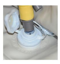
To inflate your boat, simply place the adapter into the valve and begin pumping with your foot pump. When you're finished, close the outer cap of the valve.
