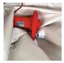
No extra nozzles are needed to inflate the main air chambers of your boat, just insert the pump into the valve and switch it on. Do not drop or suddenly move the pump while it is switched on.
