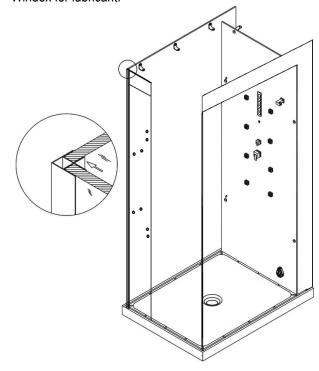
14. Assemble the half-moon shaped seals on the sides A, and C of glass D (top), if needed. See illustration below. Attach angle brackets to glass panel D. Note: The fan and speaker side of the glass will hang over the main control panel side. Place glass D (top) on the top of the unit, align connecting holes with glass D to glass panels A, B, and C. Use connector bolt to connect. Please refer to illustration below.
