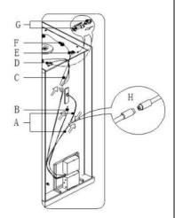
connect the light, fan and radio. Then locate the middle water pipe, which is under the faucet, and connect it to the steam box water inlet. Secondly, connect the black foam steam line, which is on the side of the steam box, to the steam outlet. Connect steam box drain line to the steam outlet drain. Finally, connect the cold and hot water lines to the water manifold, the red one is for hot water, while the blue is for cold.
