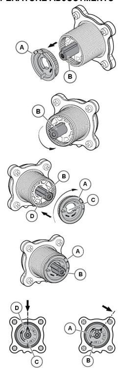
Adjustment gear (A) is factory-set to prevent stem from reaching full hot position. To adjust stem rotation: remove adjustment gear (A). Rotated steam (B) counterclockwise to determine a maximum desired temperature. Replace gear aligning adjustment stop (C) to stem tab surface (D) to stem (B) cannot move beyond adjustment point.
