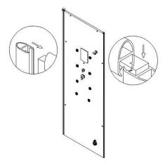
7. Install angle brackets over the installation holes of glass A, connect with connector bolts (make the connection snug, but loose enough to make adjustments.)
