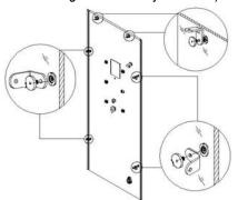
Place bottom edge of glass A into the slot on the base as shown. A small amount of soap or lubricant on the gaskets will help with installation.
