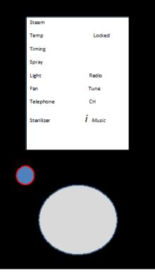
To control the music Volume with the Keypad, Highlight the *i* MUSIC, PRESS the Shuttle Knob. Press the Speaker button on the bottom left of the keypad and the dB on the display will flash, rotate the Shuttle Knob to the desired volume, press the Shuttle Knob to set.
