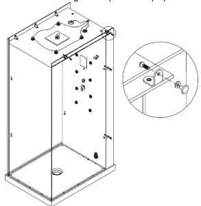
13. Place glass C into the slot onto the base and insert into the corner seal of glass B. Note: Glass C is the clear panel, and glass B is a black/white large solid panel. Line up the installation holes and connect glass B and glass C. Note: Use Windex for Jubricant.
