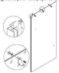
Insert the half-moon shaped rubber seals on both sides (outside facing edge), and top edge of glass A. Note: top gasket may be already installed on the control panel.
