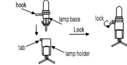
Fig. 2 Replace with the spare lamp
