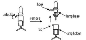
Fig. 1 Unlock and remove the burned out lamp
