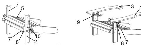
STEP 4 Put together the chair seat (5) with the backrest (6) then tighten with bolts (9), the chair arm (3) and (4) with the backrest (6) then tighten with bolts (9).
