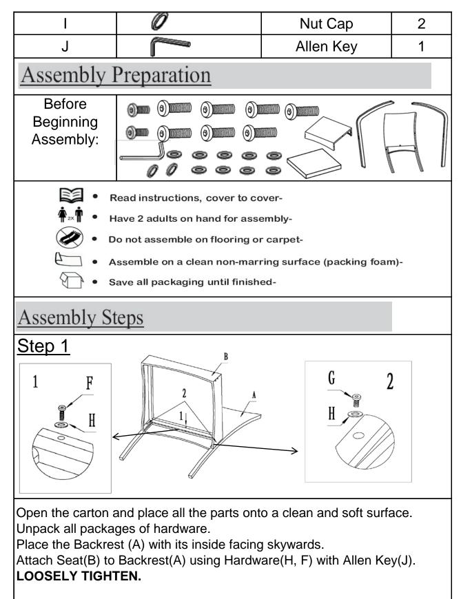
ATTENTION: Occasionally some of the PE Wicker shifts and covers the mounting positions preventing easy assembly. The PE wicker should never be cut, but moved away from the mounting positions.
