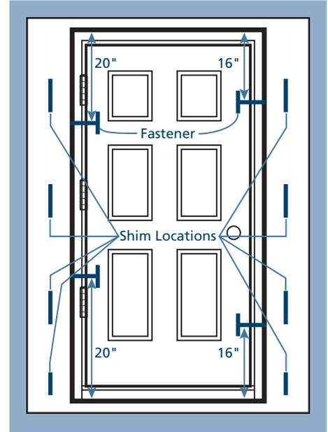
4. From the inside, shim the jambs as follows: One shim on each end of the sill (between jamb and sill, not under sill). Single/double units at each hinge location and at the strike plate. Units with sidelites, between the sidelite and wall in at least 3 places until the door is square in the opening.
