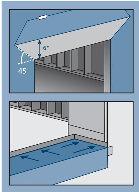
6. Cut two pieces of self-adhered flashing 6" wide by the sill pan width + 3" long.
