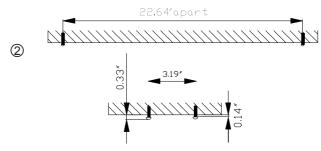
3. Lift the fixture and line up the four mounting slots on the bottom to the screws. Slide it towards the side with the power cord to secure it into place (In the case shown in Figure 3, slide to the right since the power cord is on the right side).
