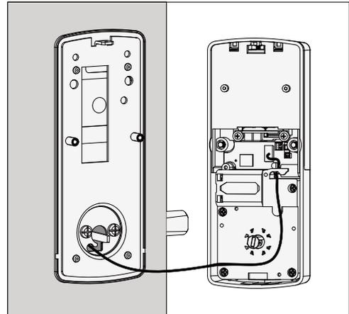
**4.6:** Before placing the interior assembly to the mounting plate, ensure the thumb turn is vertical.
