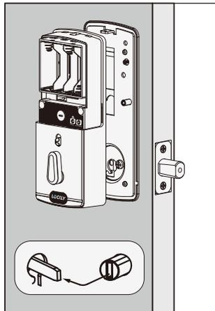
**4.8** Secure the interior assembly with 2 screws (I)
