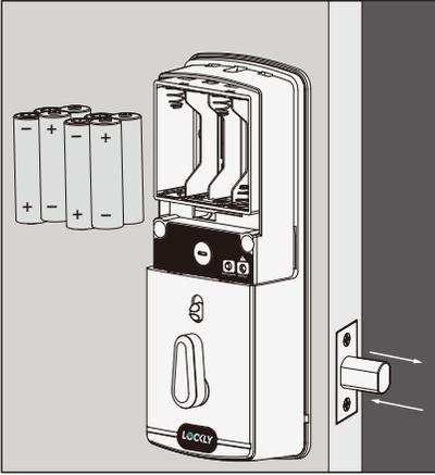
**5.1:** First install 3 of the 4 batteries. Before installing the last battery, press and hold the PROGRAM button
