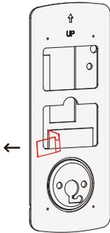
**4.1:** Peel off the cover from the adhesive strip on the mounting plate.
