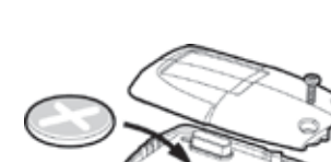
Lithium battery CR-2032 included. (Positive side up).
