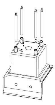
Step 2. Tighten each Set Screw using 5/32" Allen Wrench included with your sink
