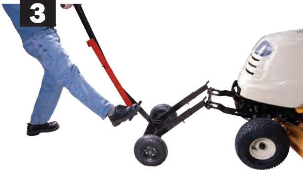
A. Apply slow continuous pressure to foot bar while bringing the handle towards the ground. B. While applying pressure with foot, bring the handle slowly towards the ground.
