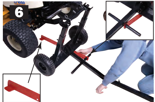
Slide stabilizer bar off footbar. Replace wingnut. Rotate stabilizer bar so stabilizer bar foot pad is resting on the ground. Slide stabilizer bar back onto footbar. Stabilizer bar should properly be in place under the tractor.
