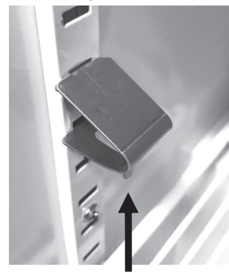
Improperly Installed Clip
