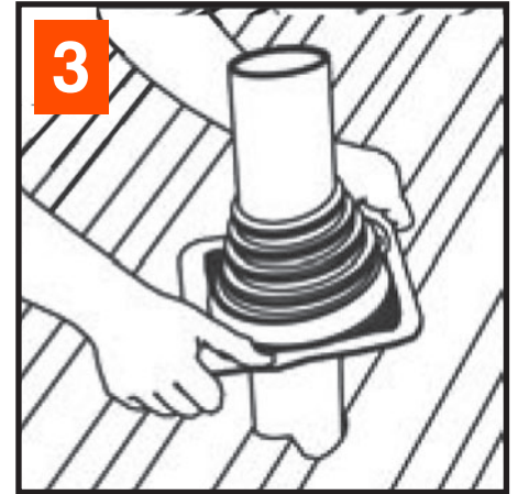
Slide flashing over pipe using water
