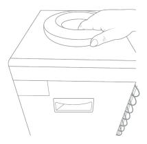
2. Put the mixture into the machine's cold tank and make sure the water can flow out of the hot water spout (#9).
