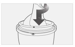
Note | The juicing screw needs to be locked in place in order to close the drum lid.
