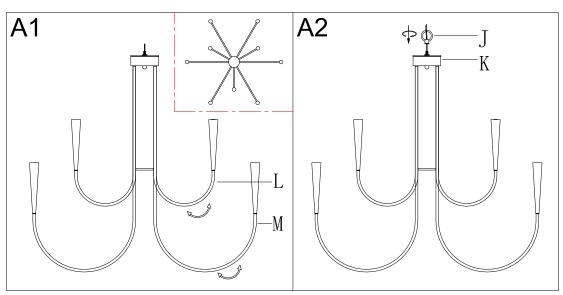
Step A1 » Adjust arms ( L & M ) to the proper position as shown in the illustration.
