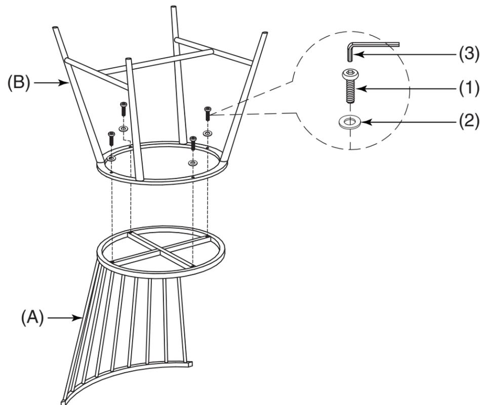
FULLY TIGHTEN ALL BOLTS USING ALLEN WRENCH (3).
