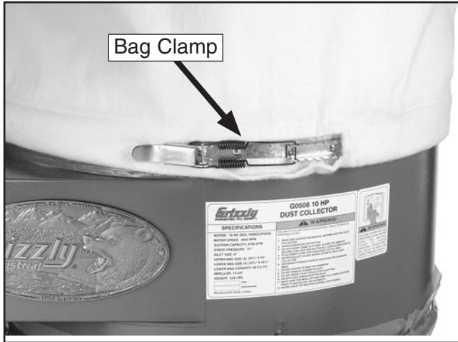
Figure 16. Upper filter bag secured to collector.
