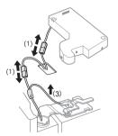
3 Rotate the hinge lever (1) clockwise. Lift the top hinge (2) free of the hinge lever latch.
