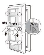
2 To replace the Door-in-Door case, line up the tabs on the Door-In-Door case with the slots on the door and push down until it snaps into place.
