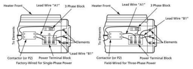
**Figure 4a** - Wiring Connections for Single-Phase and Three-Phase Power (DR-P275 and DR-P2100)
