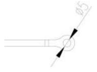
DR-P2100, DR-P275, DR-P3150 and DR-P3200 use grounding lug to install the grounding wire. The ground wire AWG# and the lug screw size of model DR-P2100, DR-P275, DR-P3150 and DR-P3200 is as below list:
