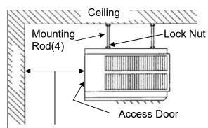
Clearance Equal to Depth of Heater to Permit Full Opening of The Access Door
