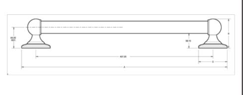
MATERIALS: Grab bar is constructed using 1-1/4" diameter 20 gauge 304
