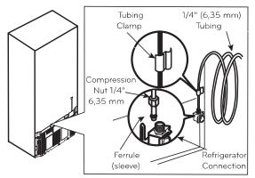
Hold on to the pipe from the handles or grabbers located behind the refrigerator, loosing first the bolt holding the handle. Afterwards, insert pipe into the hole and tighten bolt to finalize.
