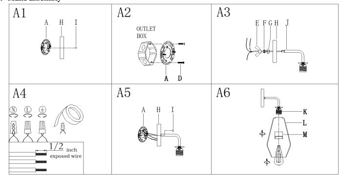
Step A1: Unscrew the knob balls (I) from the back plate(H) then gently remove the mounting plate (A).
