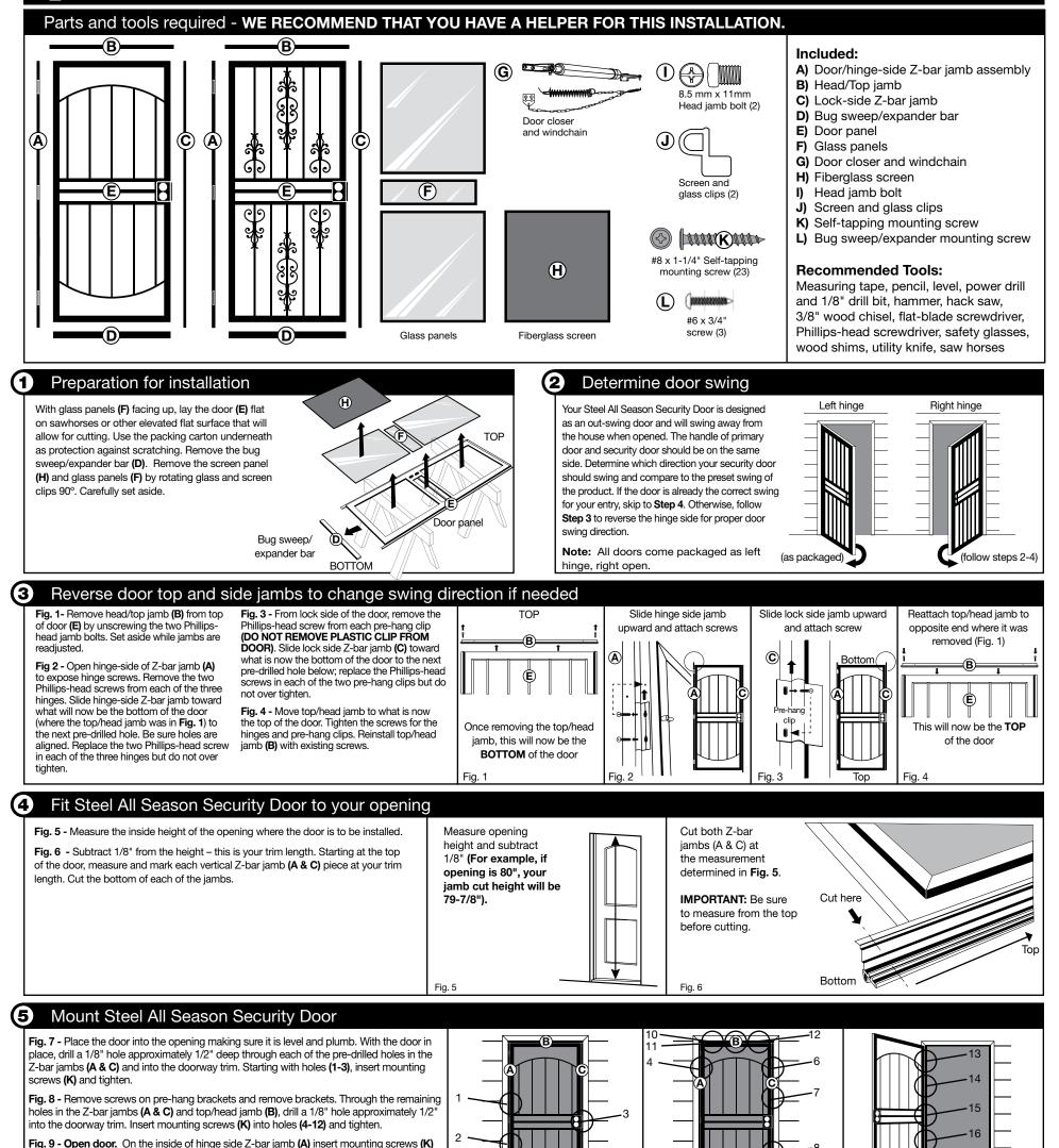
into holes (13-17) and tighten. Lastly, re-install glass and screen panels (F & H) and secure with glass and screen clips in proper position. Close and open door to ensure proper fit, adjust if necessary.
