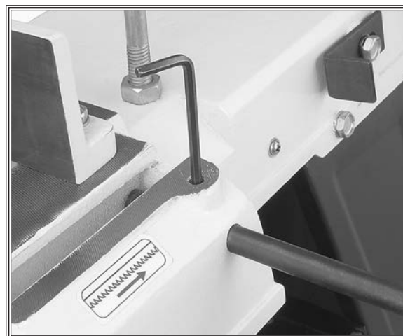
Figure 17. Installing the work stop shaft.
