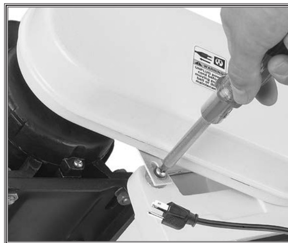
Figure 13. Installing the pulley cover.
