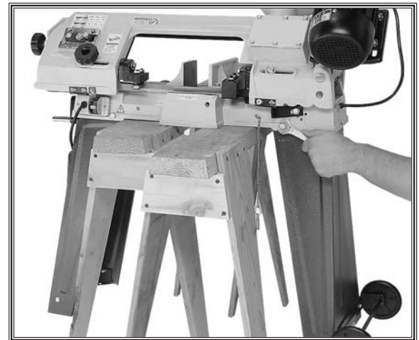
Figure 11. Attaching leg assemblies.
