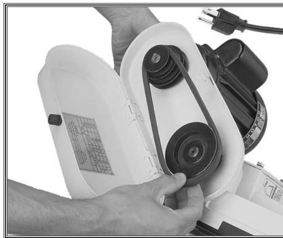
Figure 52. Installing the V-belt.
