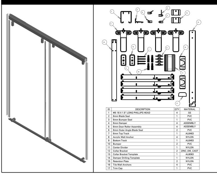
MATERIAL: Anodized Aluminum Extrusions (Track) and Zinc Die Cast (Mounting Brackets). Bronze Finish and Matte Black are Powder Coated.
