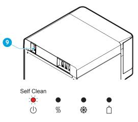
The power indicator light on the front of the dispenser will begin blinking, indicating the cleaning process is underway.
