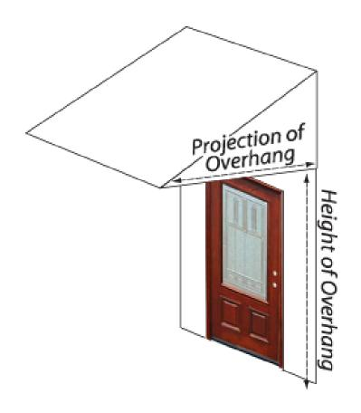
Lack of proper overhang will void warranty! Overhang must project a <u>minimum</u> of 1/2 the height of entry.
