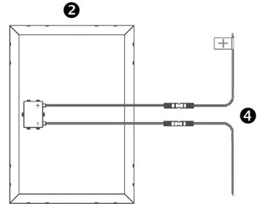
**6** Connect the bare wire end of the positive cable **4** to the “SOLAR +” input of the charge controller **1**. Connect the negative bare end to the “SOLAR -” input. Now, you can mount the GS-PWM-20A charge controller to an indoor wall or within a NEMA-3R rated enclosure.
