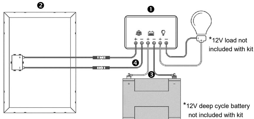
**7** Remove the panel covering. In good sunlight, the charge controller's **1** "BAT %" should increase to 100%. Once the battery is fully charged and the controller is set to "LOAD ON," the system will provide power through the load control output or through the two USB ports. If an inverter is added to the system, it must be connected to the battery bank, and not to the charge controller.
