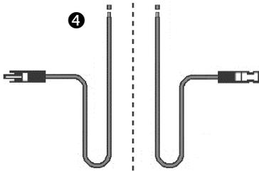
**5** Connect the MC4 ends of the halved cable **4** to the compatible MC4 ends of the solar panel **2** cables. (Mark the end of the positive panel cable with a piece of tape to help distinguish polarity during connection.)
