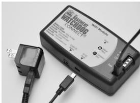
5. The red and green lights on the WiFi module should start alternating
