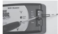
WiFi module. Turn the screw clockwise to secure the wire.
