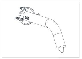
Remove the two retention screws and remover the body from the base. Drill 3/16" holes on the marks and insert anchors. Attach the base to the wall using the supplied screws
