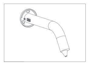
Feed the soap tube and sensor connector through the wall and reattach the body to the base by tightening the retention screws.
