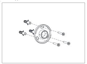
Reinstall the escutcheon by threading it clockwise onto the base.
