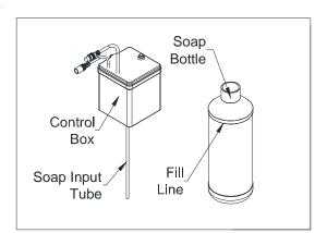
2. Re-attach the soap bottle to the control box, making sure that the soap input tube is inside the soap bottle. Depress the green system prime button until soap comes from the nozzle. The system is now ready to
