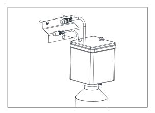
4. Push the soap tube onto the outlet connection on the control box. Secure the tube with the clamp.
