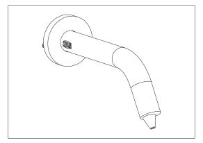
Note: It is recommended to horizontally offset the soap dispenser spout with the faucet 4 - 6" and to install vertically 6-10" above the sink drain at the same height as the faucet. To comply with ADA standards, the center-point of the soap dispenser spout must be less than 50" from finished floor.
