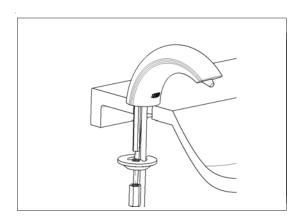
2. Ensure that the mounting adapter is oriented as shown, with the soap tube and sensor connector running through the cutout. Tighten the mounting nut.
