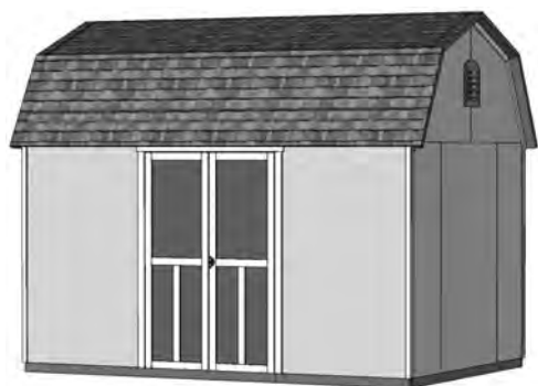
OPTIONAL: DOOR LOCATED ON EAVE WALL
