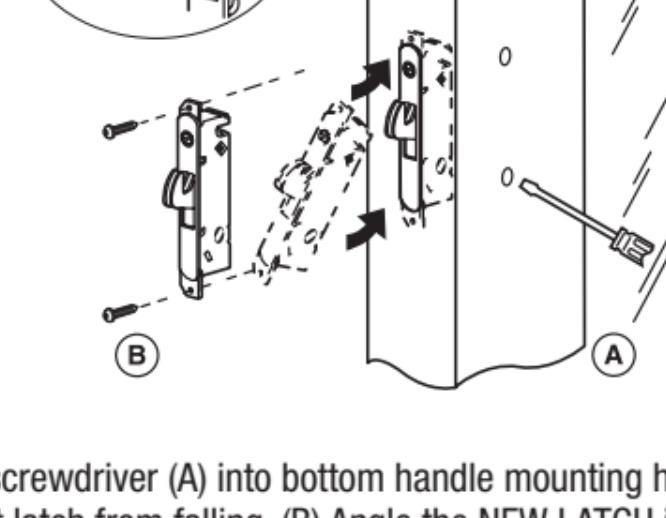
Insert screwdriver (A) into bottom handle mounting hole to prevent latch from falling. (B) Angle the NEW LATCH into position and hold securely to prevent it from falling down the stile. **NOTE: To ensure the latch will not fall into the stile, wrap string around the extended hook and tape securely (C), Anchor string to a heavy object to allow free hands for attaching latch in position.** Reattach mounting screws and tighten securely. Reattach patio door handle. Check for proper operation.
