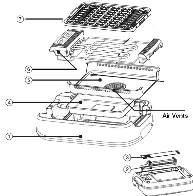
First, Turn the appliance over , put the fan motors at the bottom see Part 1. 2. 3.
